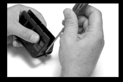
**Step 4**) Using light pressure pry retaining bar out. Repeat steps 4 and 5 until bar can be removed by hand.
