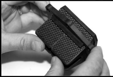
**Step 1b)** For reed valves with short reed stops, no tool is needed, push cage firmly through manifold as shown.
