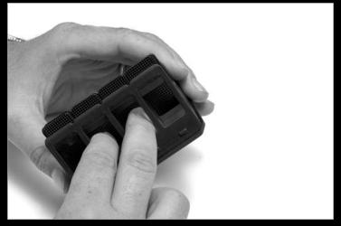
**Step 5**) With retaining bars removed, push reeds free of locating tabs (as photo illustrates) now reeds can be removed.
