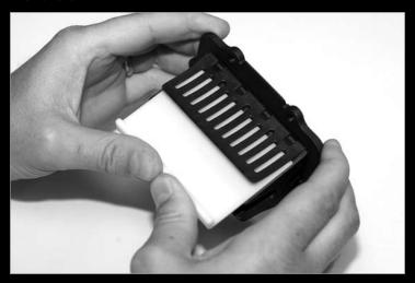
**Step 1a)** For reed valves with extended reed stops, insert tool between reed and reed stop and push cage firmly.
