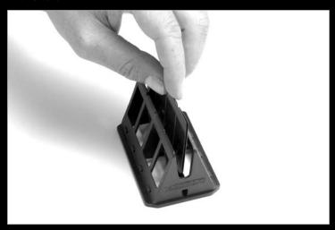
**Step 6)** Place two reeds in center of reed cage, making sure they are at the bottom.
