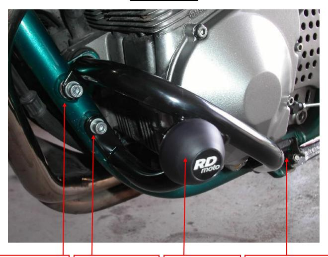
bolt M8x60mm + pad M8 (spring) bolt M8x70mm + pad M8 (spring) crash protectors with the logo RDmoto is not included in this type of crash bar bolt M10x60x1,25mm + pad M10 (spring)
