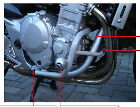
steel bolt M10x240mm + two pads M10 + two nuts M10
