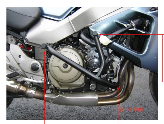
Insert dural.cylinder between the fairing and frame ,use bolt M10x85 + plastic plug into the tube 22mm
