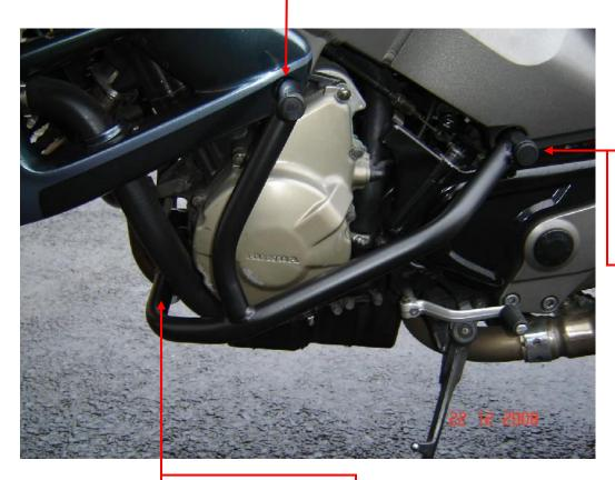
steel bar d=335mm + steel nut M12 + plastic plug into the tube 25mm
