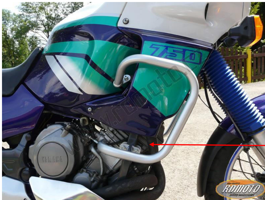
steel adapter with thread M8 + two bolts M8x40mm + two nuts M8 (safety)
