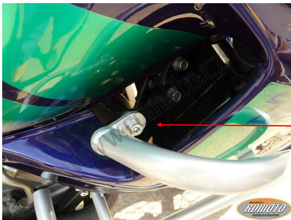
bolt M8x25mm + two pads M8 (plane) + nuts M8 (safety) + steel adapter (bent)
