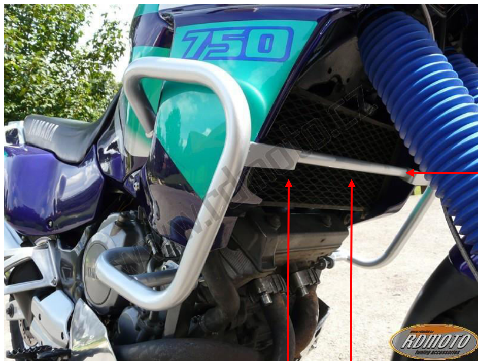
bolt M8x25mm + pad M8 (plane)
